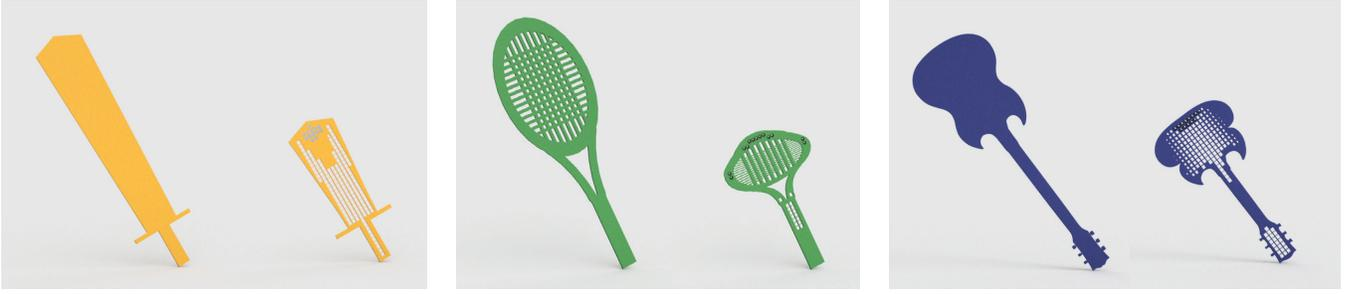
Figure 10: VR controllers designed with our system: Sword (Left), Tennis racket (Center), and Guitar (Right). For each pair, the target virtual object is shown in the left, and the designed controller is shown in the right.
