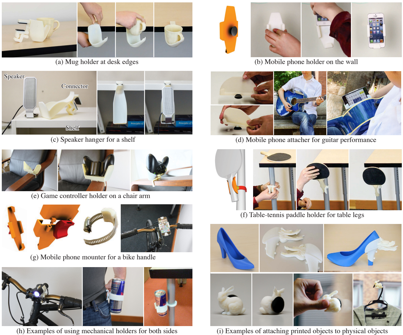
Figure 13: Applications of AutoConnect. In examples (a)–(g), we connect a structured object and a free-form object. Our method can also be used for other cases such as (h) the case that both objects are structured, and (i) the case that one side is directly printed.
